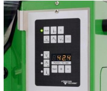
**Fig. 2:** Control unit with 7-row display
